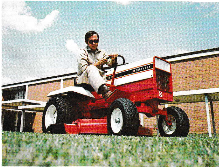
Gravelly 812, 12 HP Riding Tractor with 50-inch Center-Mount Rotary Mower
