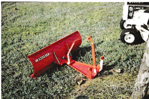
Move snow or do light grading with this 42-inch SnowDozer that attaches to your 408 in just minutes. Keep old man winter off your walks and drives all winter long!
