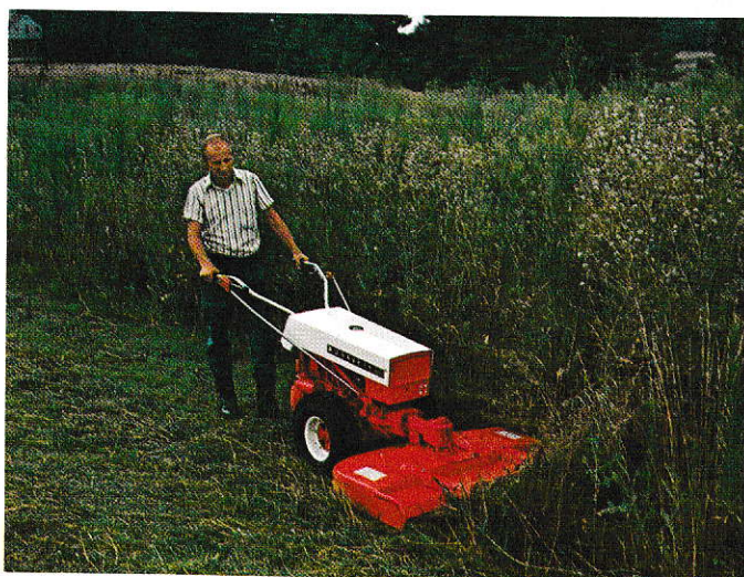
Gravely 12 HP Convertible Tractor with 40-inch Commercial Rotary Mower—Rough Mowing
