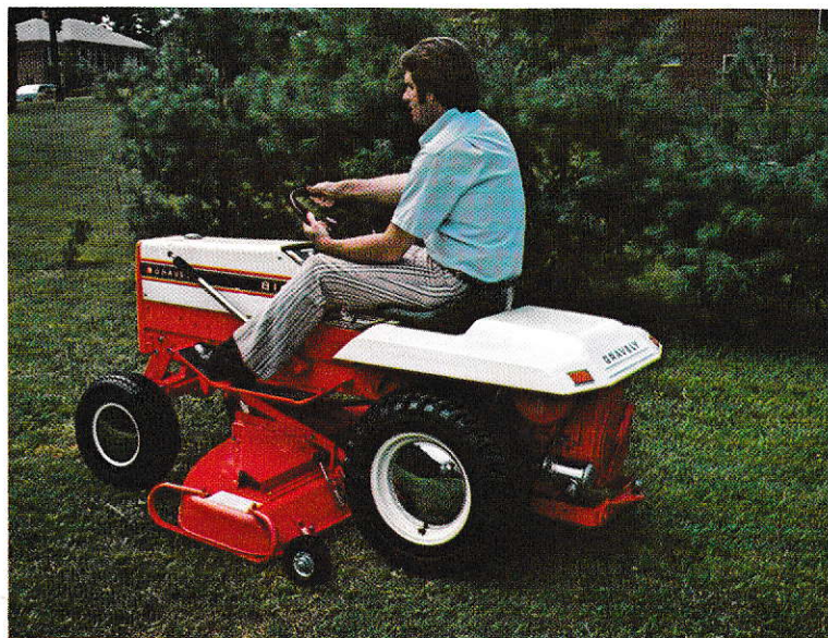
Gravelly 810, 10 HP Riding Tractor with 50-inch Center-Mount Rotary Mower
