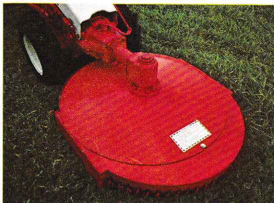
30-Inch Rotary Mower and Optional Chain Guard.
