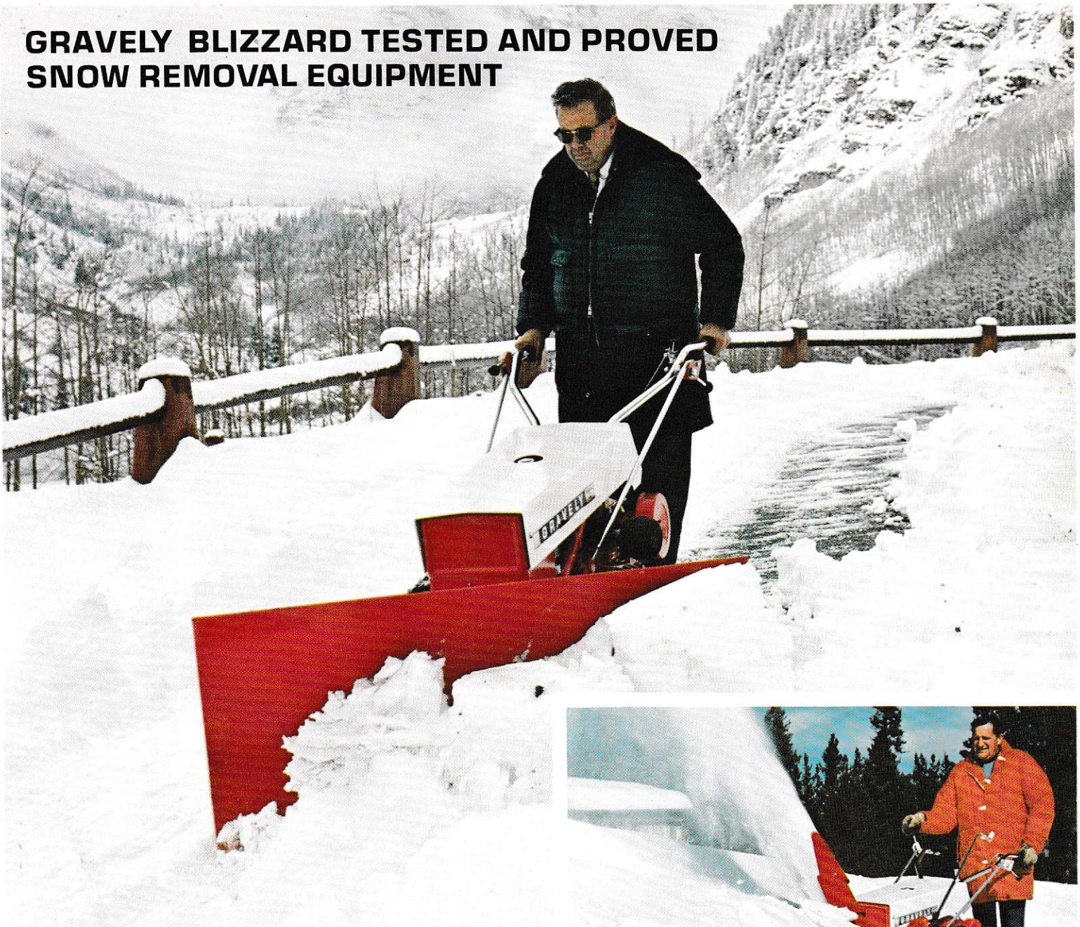
Gravelly 12 HP Convertible Tractor with 48-inch SnowDozer
