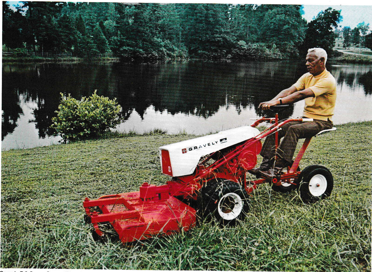
Gravely 7.6 Super Convertible with Optional Dual Wheels, Steering Sulky, and 40-inch Commercial Rotary Mower
