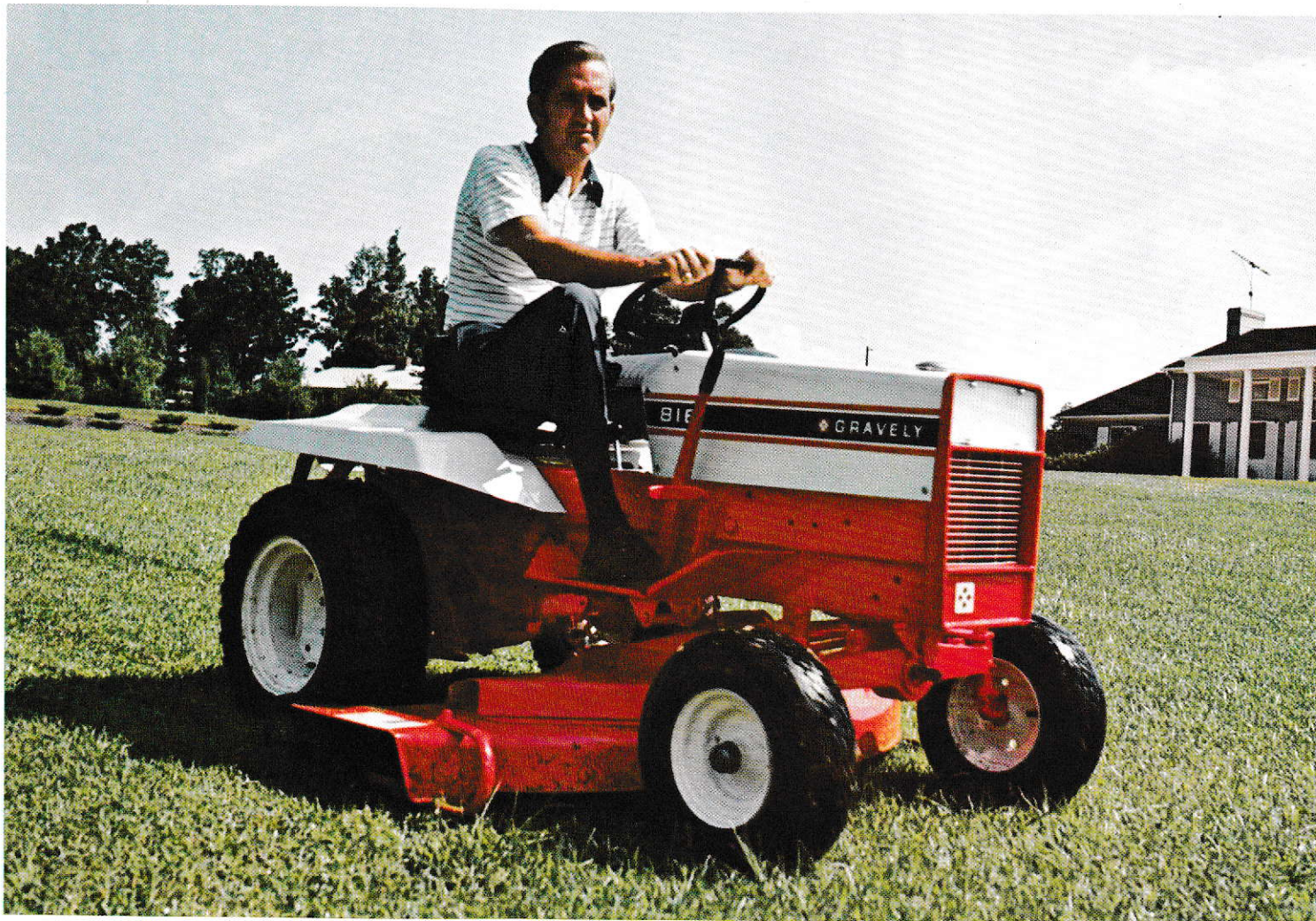
Gravely 816 Riding Tractor with 50-inch Rotary Mower
