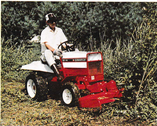
Gravely 814, 14 HP Riding Tractor with 40-inch Commercial Rotary Mower
