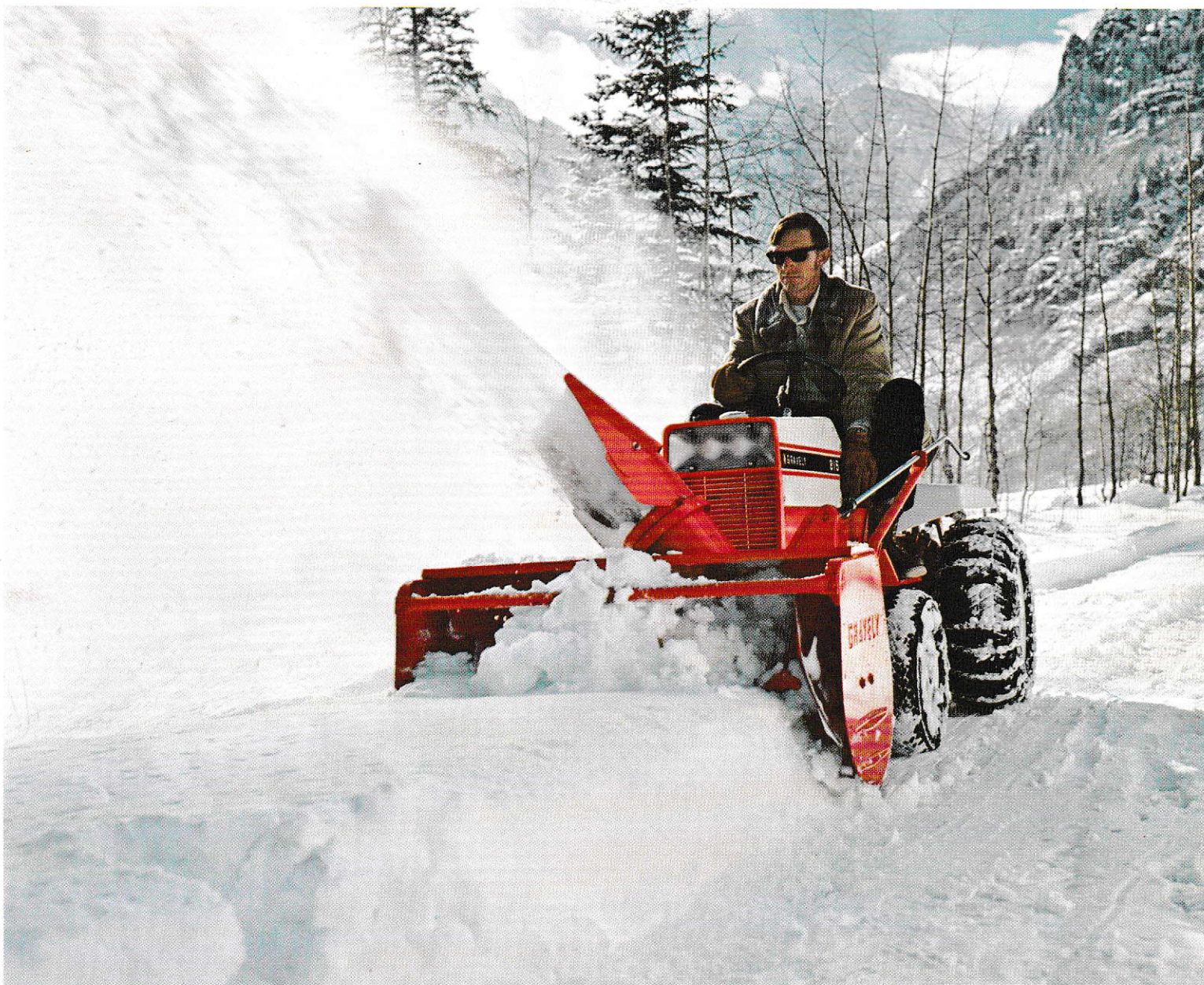
Gravelly 816, 16.5 HP Tractor with 44-inch Snowblower
